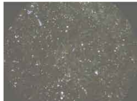
Figure 21. Arachidic acid film in silicon wafer (Optical microscope, 50x, dark field)
