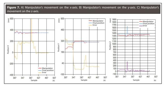
tory described by the joystick device, thereby reducing error as the manipulator approached the final position and validating the machine vision system's effectiveness.
