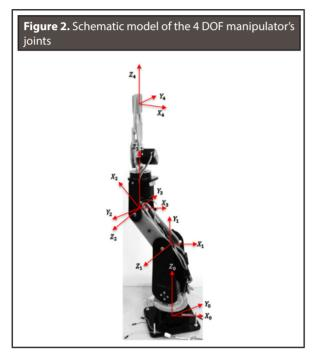
These servomotors have a rotation range of  $0^{\circ}$  to 135° with a torque of less than 6.91 kg-cm. In accordance with these characteristics, the manipulator's workspace depends on the position in which these motors were situated and the mechanical tolerances, as well as the form and the material. **Table 1** shows the turning range of each of the robot's joints.
