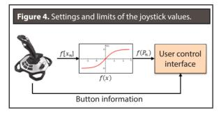
The settings data are multiplied by a conversion factor which depends on the robotic arm's forward speed and the joystick's sampling period. Based on the tests performed, the conversion constant and speed  $k_v$  is 2.2. The robotic arm's movement matrix to calculate the manipulator's new position is represented by **Equation 11**, which shows a point-to-point sequence to follow the manipulator's trajectories.
